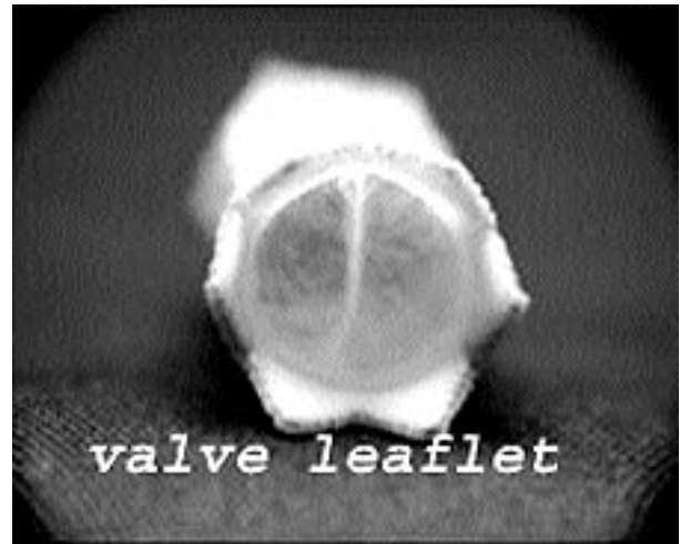
Fig. 9. Bovine jugular vein mounted on nitinol stent. Courtesy of VenPro, Irvine, CA.
